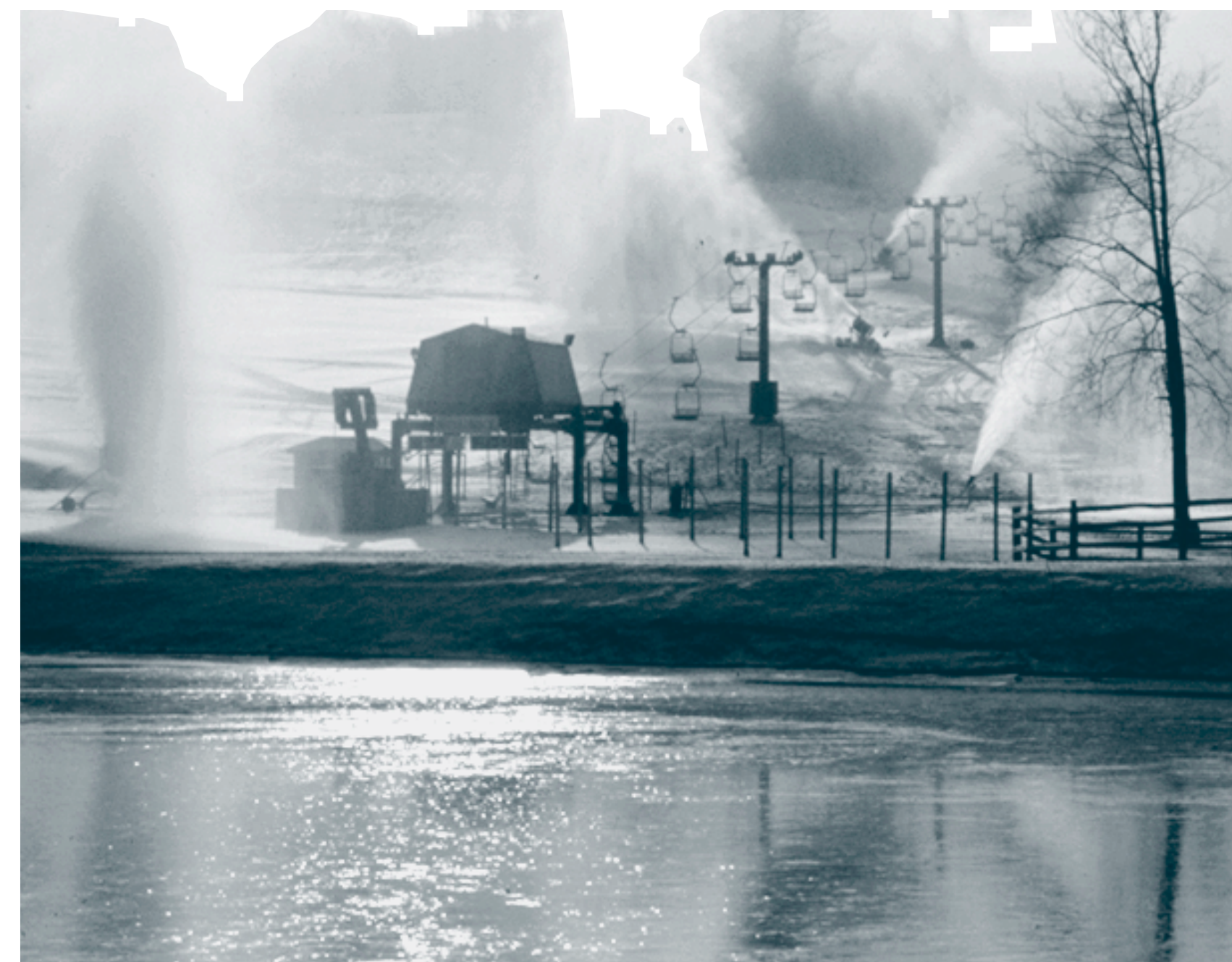
SNOWMAKING AT WACHUSETT IS A SIMPLE PROCESS THAT CALLS FOR THE SAME BASIC INGREDIENTS AS NATURAL SNOW – WATER AND AIR.
